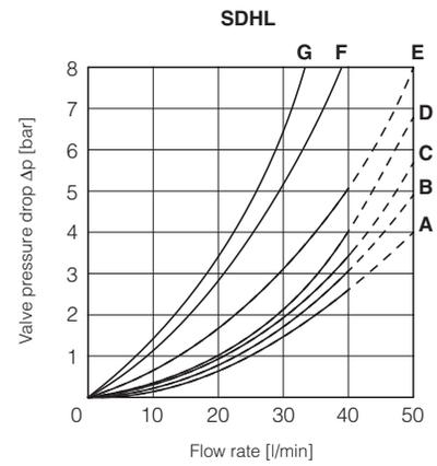
**9 OPERATING LIMITS** based on mineral oil ISO VG 46 at 50°C
